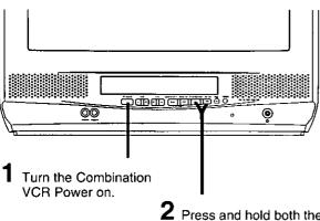
Press and hold both the PLAY and FF on the Combination VCR for more than 5 seconds.
